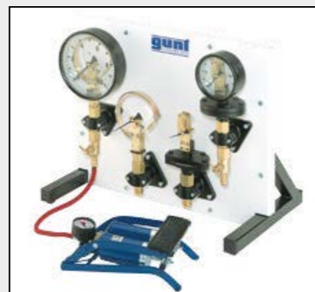
left: HM 700.15 Various Screwed Pipe Connections LxWxH: 500 x 370 x 400 mm Weight: approx. 15 kg Item No. 070.70015
