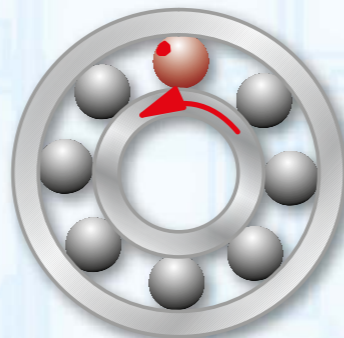
A damaged rolling ball element, frequency 4,65 \Omega
