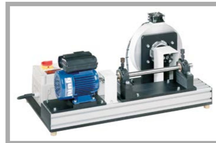
The illustration shows MT 172 together with the journal bearing-supported shaft MT 170.
