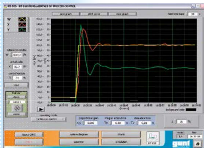
Control behaviour of a PID controller with non-optimised adaptation of controller parameters
