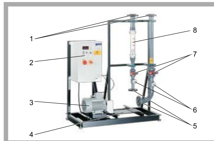
1 flange connections to connect HL 962 to HL 962.30, 2 switch box with displays and controls, 3 electric motor, 4 mounting plate for test pump, 5 flange connections for test pump, 6 manometer, 7 valve, 8 flow meter
