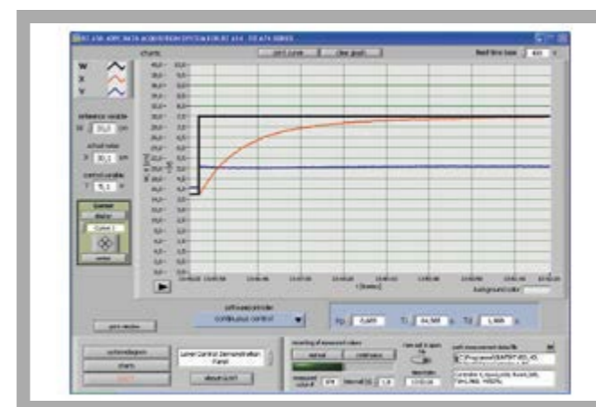
Screenshot of optional I&C software RT 650.40: step response to change in reference variable, with PID controller
