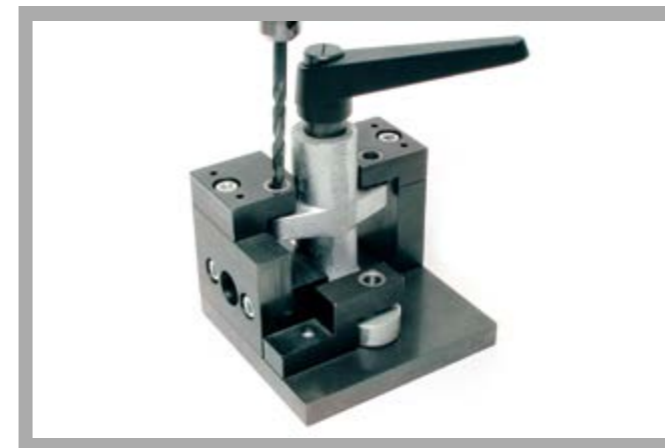
Drilling jig in use
