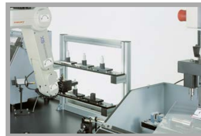
The illustration shows the robot storing a machined part on a pallet in the finished parts store
