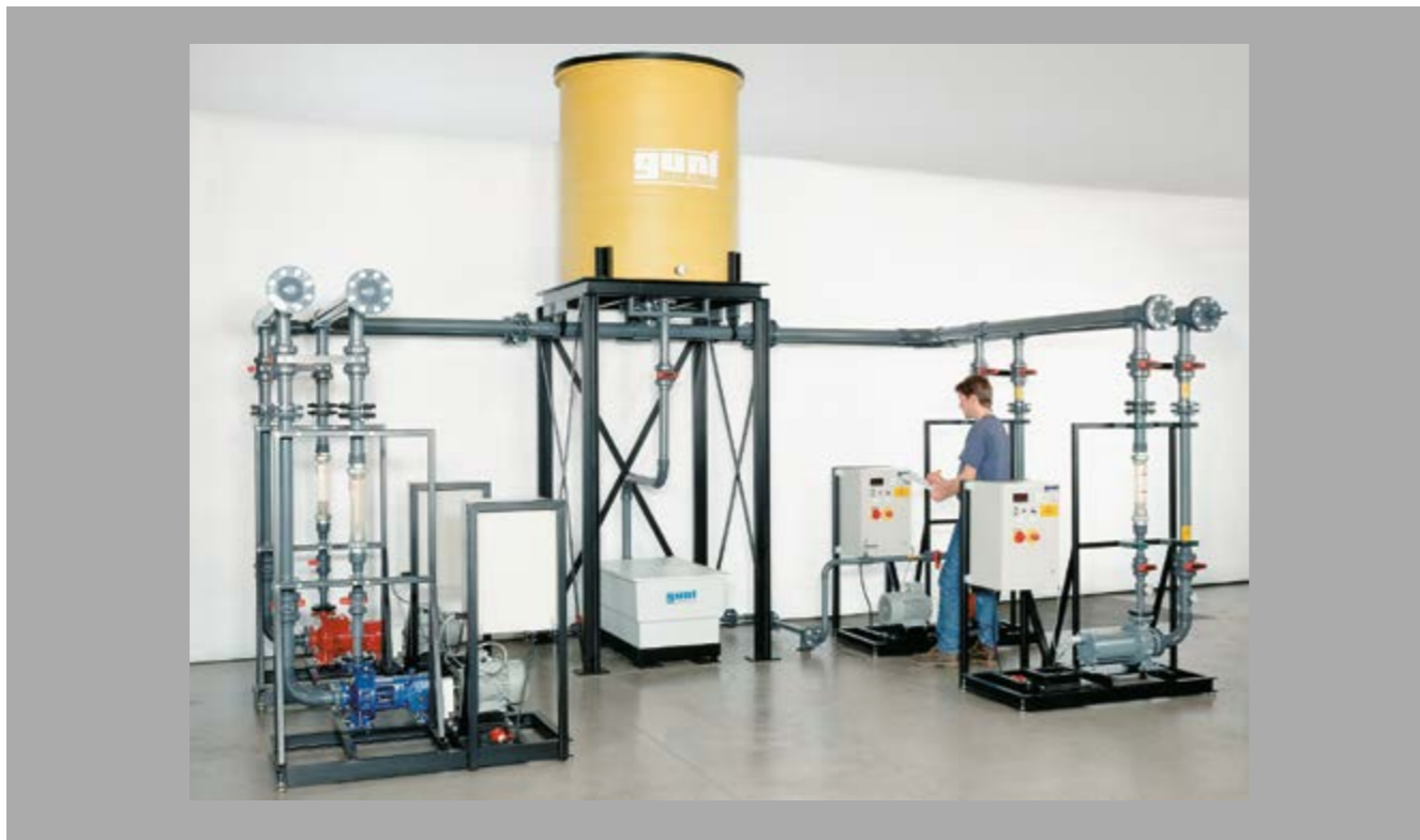
The illustration shows the complete layout of a pump system, comprising four HL 962 assembly stands, each with one pump (HL 962.01 - HL 962.04), the piping system HL 962.32 and the tank system HL 962.30.
