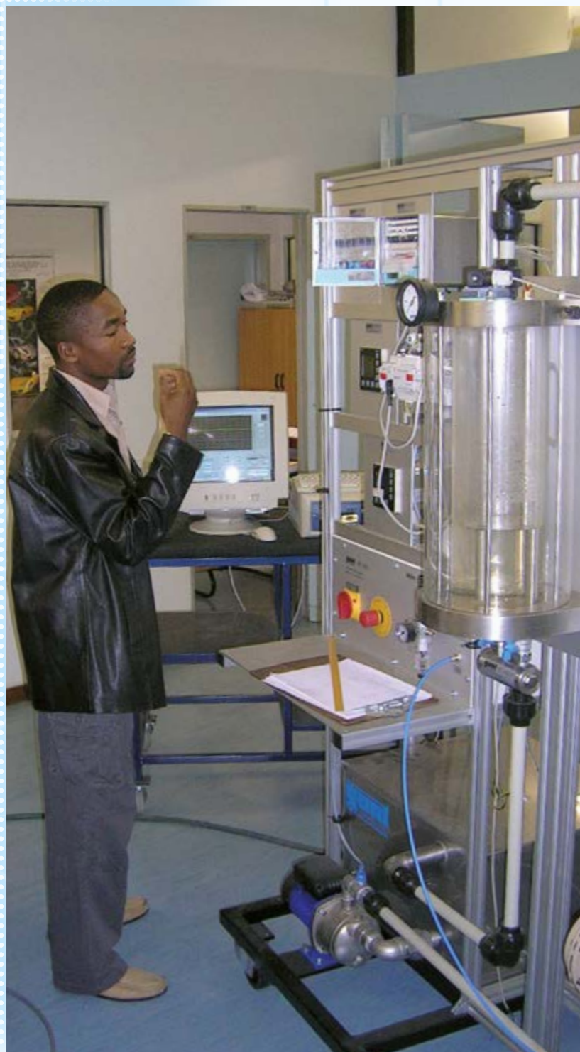
RT 450: Level control with a continuous controller or with a PLC Windhoek Polytechnic, Namibia
