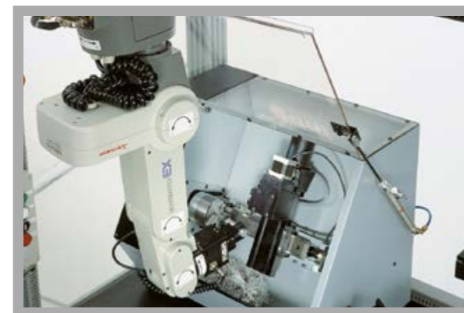
The illustration shows the robot removing a part from the lathe
