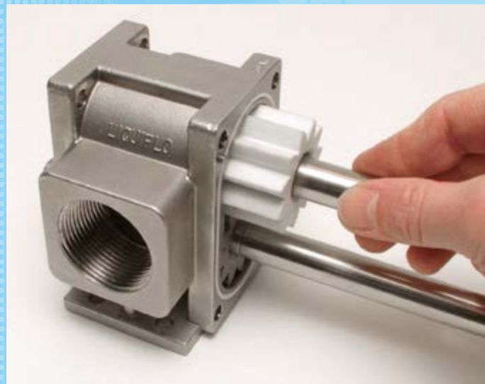
Installing the driven shaft
