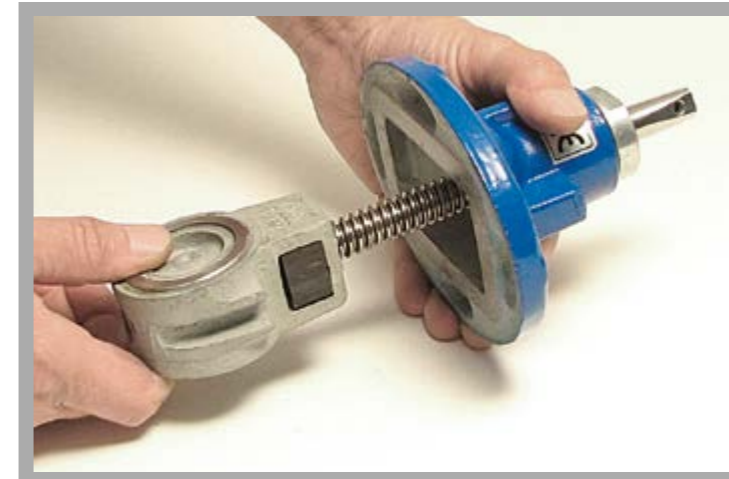
Assembly of the slider
