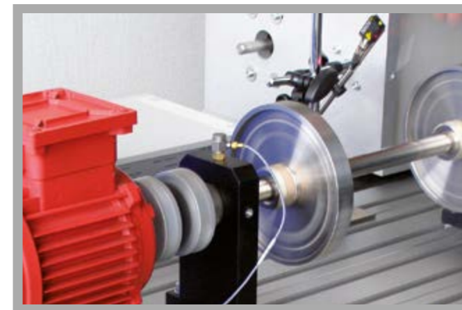
Application of the sensors: acceleration sensor on the black bearing support, speed sensor with holder
