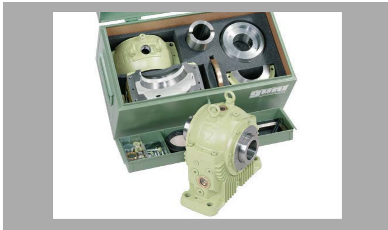
The illustration shows the tool box with parts set and tool compartment insert. A fully assembled journal bearing as is assembled from the parts is shown in the foreground.
