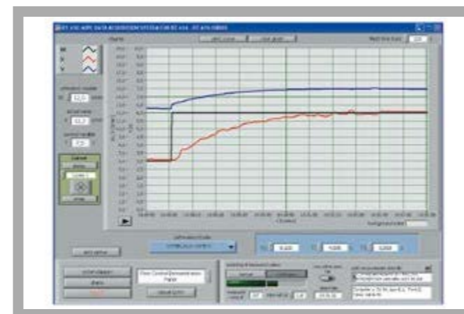
Screenshot of optional I&C software RT 650.40: step response to change in reference variable with slow PI controller
